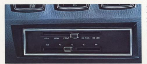
Automatic Temperature Control is standard on every Lincoln Continental. This sophisticated year-round air conditioning/heating system cools or warms rapidly to within a degree or two of the temperature you pre-select. And maintains this environment without any further manual adjustment. The air conditioner dehumidifies as it cools. Can remove pollen and dust from incoming air. At the touch of a switch, it can defog or de-ice the windshield.
