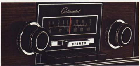
AM/FM Stereo Radio system. Includes stereo receiver, push buttons for 5 AM and 5 FM stations, 4 speakers, side-to-side and front-to-rear balance controls and a power antenna. On FM, an indicator light signals the reception of a stereo broadcast, and the system switches automatically to binaural reception. This is one of three optional sound systems for each of the Continentals.
